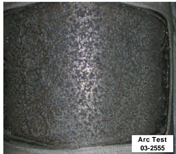
Figure 2: ARC15 Hood with Clear Shield Window After a High Incident Energy Arc Exposure
