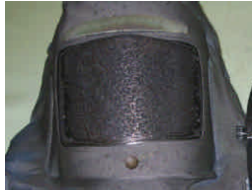
079 Clear Shield Window with UV Screener and Scratch Resistant Coating after 27.7 cal/cm 2 arc exposure
