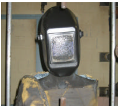
Figure 4: Auto-Darkening Window in Welding Helmet After Arc Exposure
