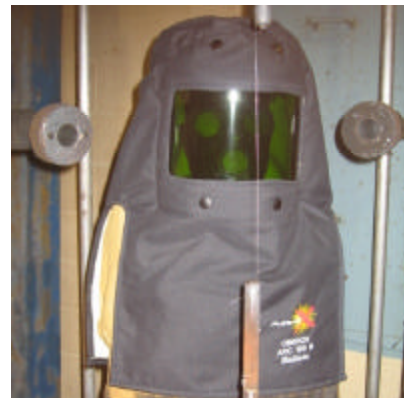
Figure 3: Auto-Darkening Window in an ARC100B Hood
