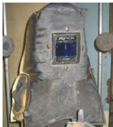
Figure 5: Auto-Darkening Window in ARC100 Hood After Arc Exposure
